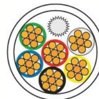
6 Core Un-screened Alarm cable with cross section diag.
